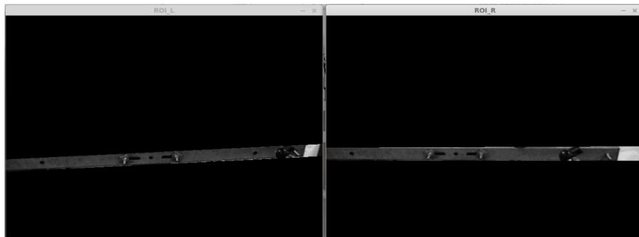
Fig. 6. Cross-arm detected and segmented.
