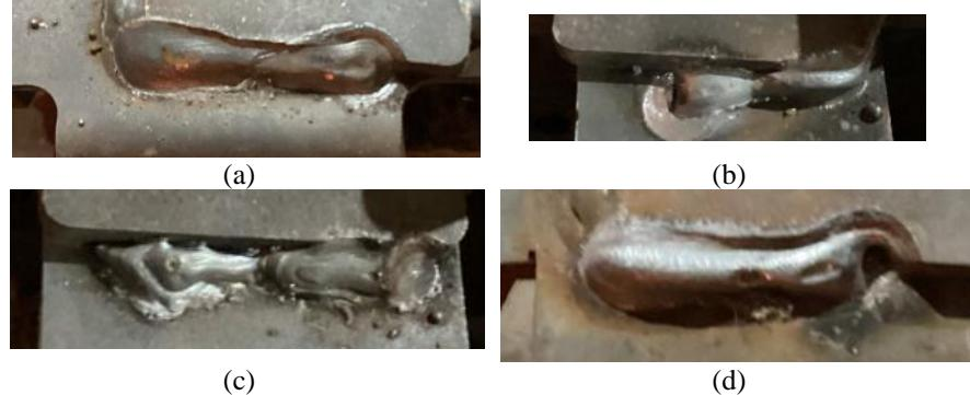
**Fig. 10.** Examples of weld seams belonging to the four categories. (a) Good, (b) Robot, (c) Human, and (d) Scrap.
