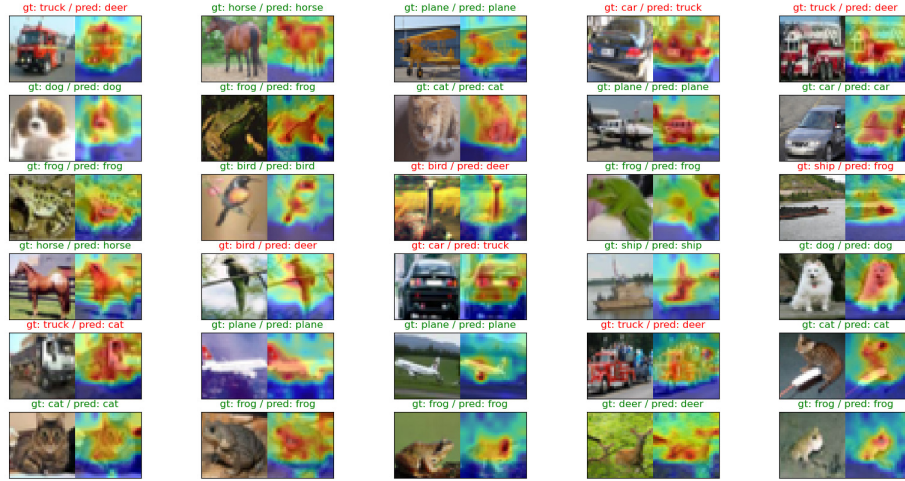
Fig. 7. Heat map generated by the ViT HAM B model's captured attention after training.
