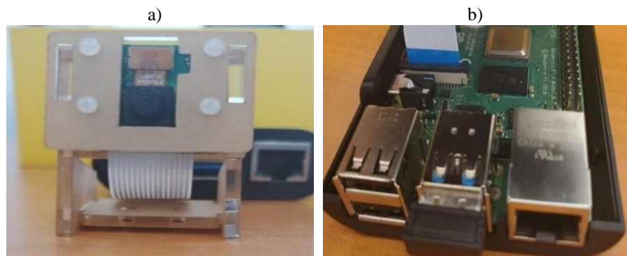
Fig. 5. a) The used Raspberry pi camera. b) The connection between the camera and the Raspberry Pi computer: The camera cable is plugged into the internal port [18].
