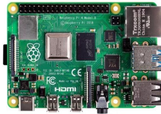
Fig. 3. The Raspberry Pi 4 model B computer.
