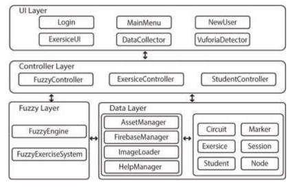
Fig. 1. CircuitAR architecture.
