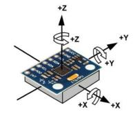
Fig. 4. Reference of position of the MPU-6050 sensor in the band.
