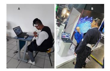
Fig. 3. A) Posture sensor placed in the vest. B) Posture sensor placed on the body band.
