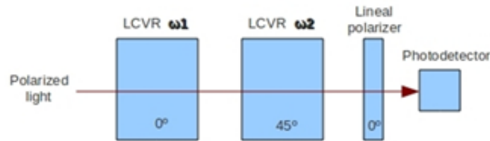
Fig. 1. The set-up for a Stokes polarimeter. The angles associated with each component refer to the relative angle of the optical axis of that component. \omega_1 and \omega_2 are the frequencies of the variations of the retardances.
