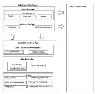
Fig. 2. SafeRoute system architecture.
