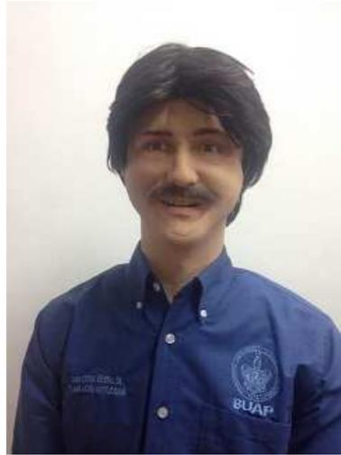
**Fig. 2.** Humanoid robot al LKE Laboratory.
