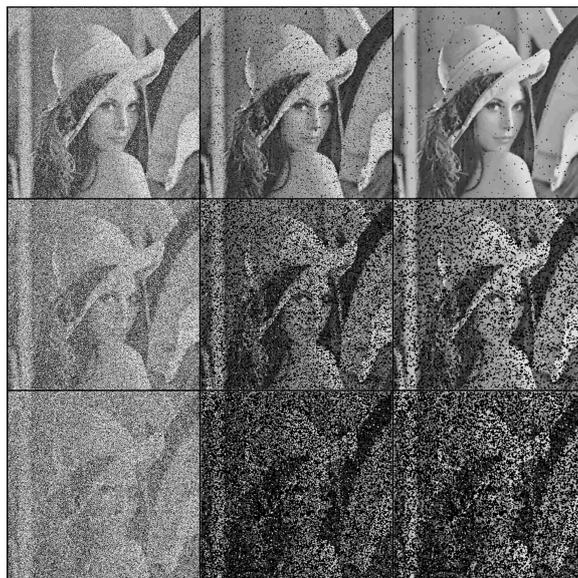
**Fig. 1.** From left to right, first row: An image with 20% of impulsive noise, opening morphological filter ( $\gamma_B$ ) and closing-opening( $\varphi_B(\gamma_B)$ ), second row: image with impulsive noise of 50%, morphological filter  $\gamma_B$  and  $\varphi_B(\gamma_B)$ , third row: image with 70% of impulsive noise, morphological filter  $\gamma_B$  and  $\varphi_B(\gamma_B)$
