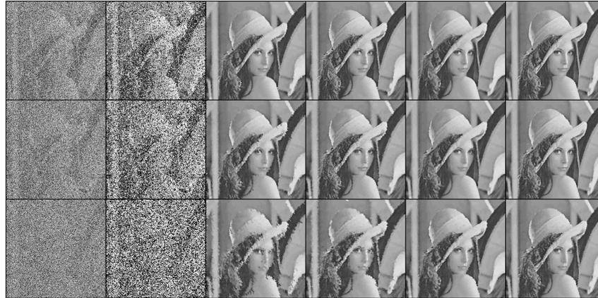
**Fig. 6.** Results of noise removal algorithms for the Lenna image. From left to right: 1st column: image with impulsive noise of 70%, 80% and 90%, 2nd column: Output of MF, 3rd column: DBA, 4th column: AMF, 5th column: NAFSM, 6th column: the proposed method
