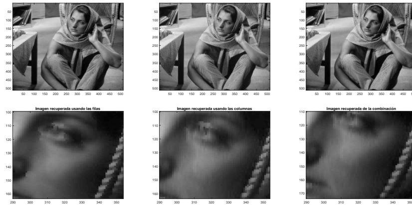
Fig. 2. From left to right: Smoothed image of Barbara after using the method on each row of the original image, smoothed image after using the method on each column of the original image, resulting smoothed image after combining the previous two
