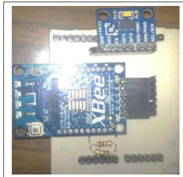
Fig. 8. Accels placed in test subject and orientation axis.
