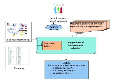
Fig. 1. Architecture of the system
