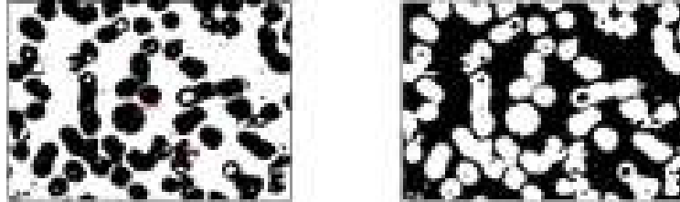
Fig. 6. Original image after adaptive thresholding (left) and (right) image after median filtering, closing and opening operations.
