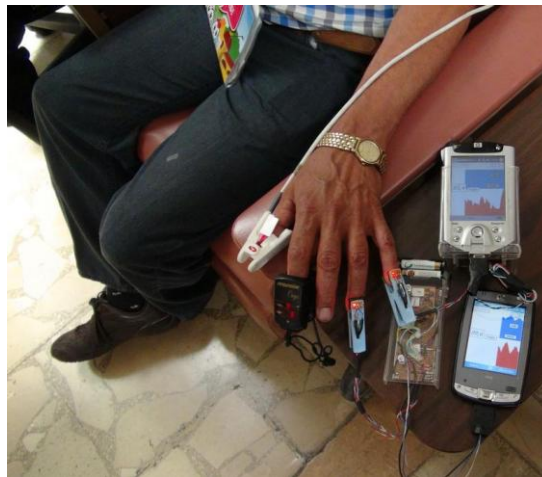
Fig. 7. Oximeters test; Mazimo, Nonin and Oximeter WiFi in a patient.
