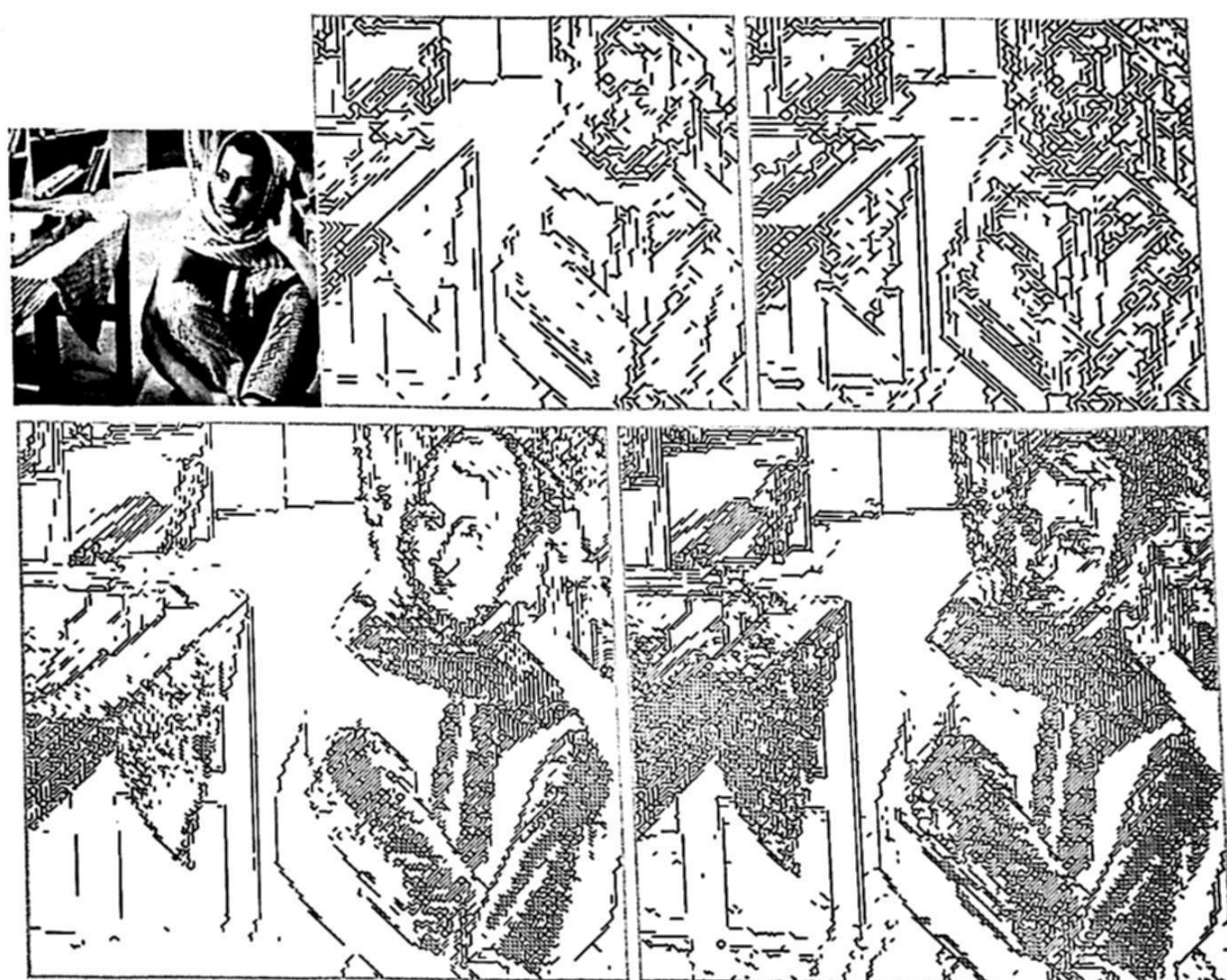
Fig. 3. Barbara images BE classified. Top left, Original. Top center and right, 8^2 blocks, d_{NE} = 20 and d_{NE} = 10 , respectively. Bottom left and right, 4^2 blocks, d_{NE} = 20 and d_{NE} = 10
