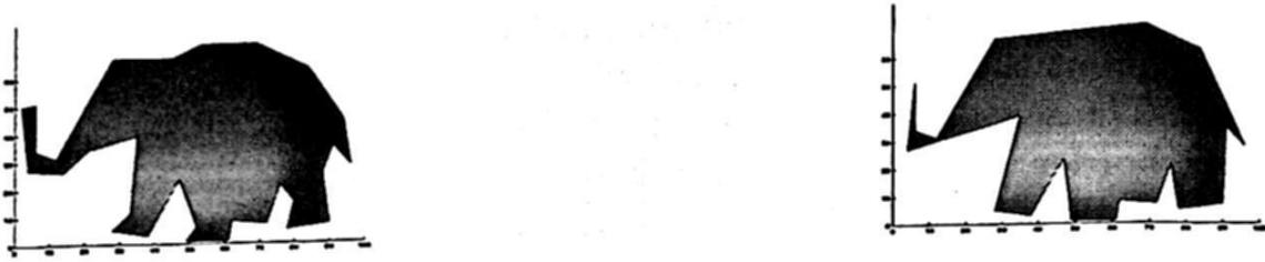
Fig. 2. The closed polygon on the left is the evolution of the original polygon, it has 30 segments. On the other hand, the figure on the right shows a stage of evolution with just 20 segments; in spite of this the main visual parts are maintained.
