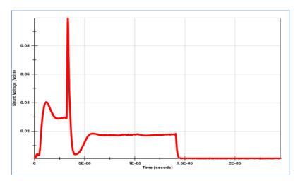
Fig. 4. Voltage across the shunt resistor.
